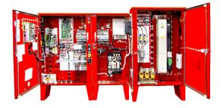
**Description** – Firetrol\* Variable Speed Electric Fire Pump Controllers provide a variable frequency drive (VFD) in a PID process control loop to control the speed of a centrifugal pump for the purpose of limiting system pressure in a fire sprinkler system. These controllers are available in the following configurations:
